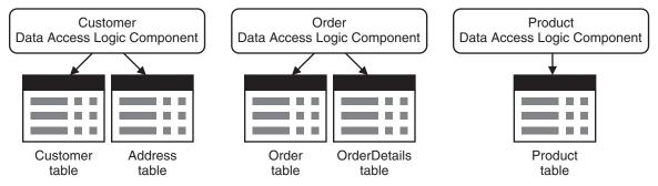
**Figure 4**Defining data access logic components to expose relational data to .NET applications
