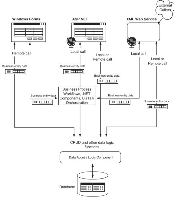
**Figure 5** *Application scenarios for data access logic components*
